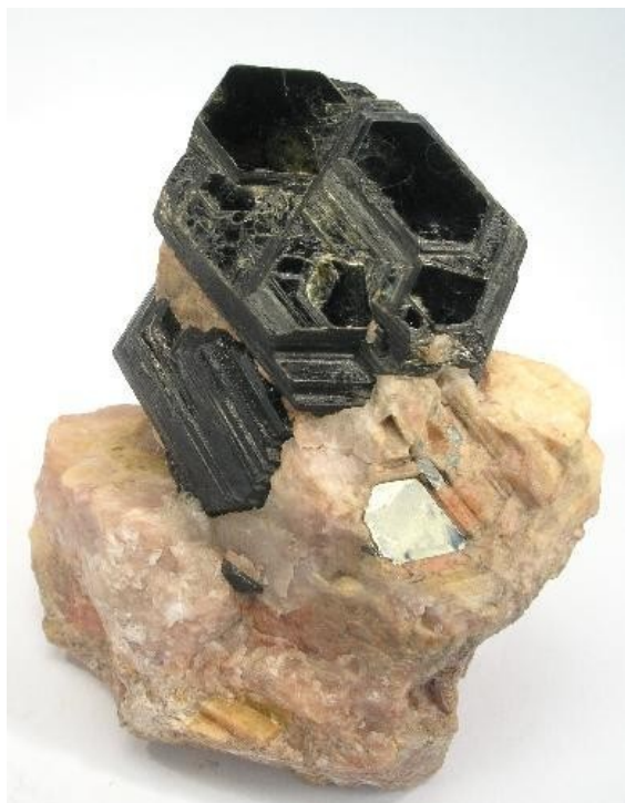
Perfect basal cleavage as seen in biotite (black), and good cleavage seen in the matrix (pink orthoclase).
