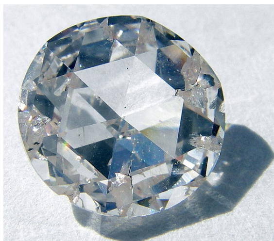
Colorless gem cut from diamond grown by chemical vapor deposition
