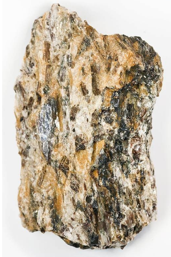
Schist is a metamorphic rock characterized by an abundance of platy minerals. In this example, the rock has prominent sillimanite porphyroblasts as large as 3 cm (1.2 in).
