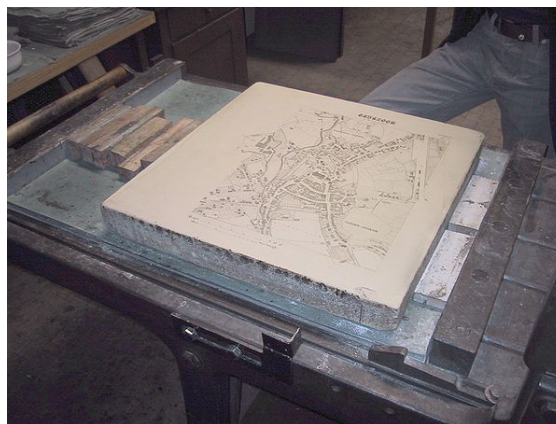
A limestone plate with a negative map of Moosburg in Bavaria is prepared for a lithography print.
