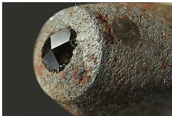
The extreme hardness of diamond in certain orientations makes it useful in materials science, as in this pyramidal diamond embedded in the working surface of a Vickers hardness tester.
