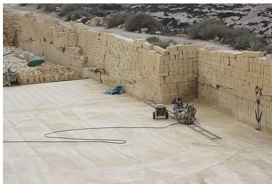
Cutting the limestone blocks at a quarry in Gozo, Malta
