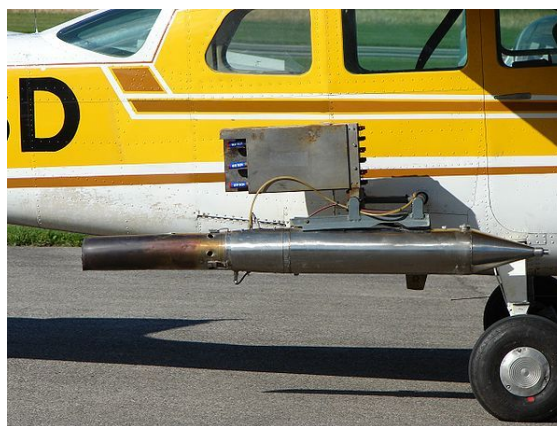
Cessna 210 equipped with a silver iodide generator for cloud seeding
