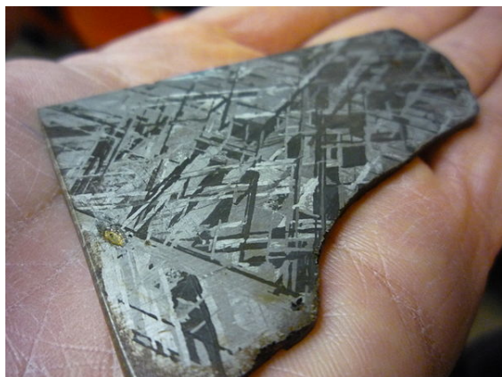
Widmanstätten pattern showing the two forms of Nickel-Iron, Kamacite and Taenite, in an octahedrite meteorite
