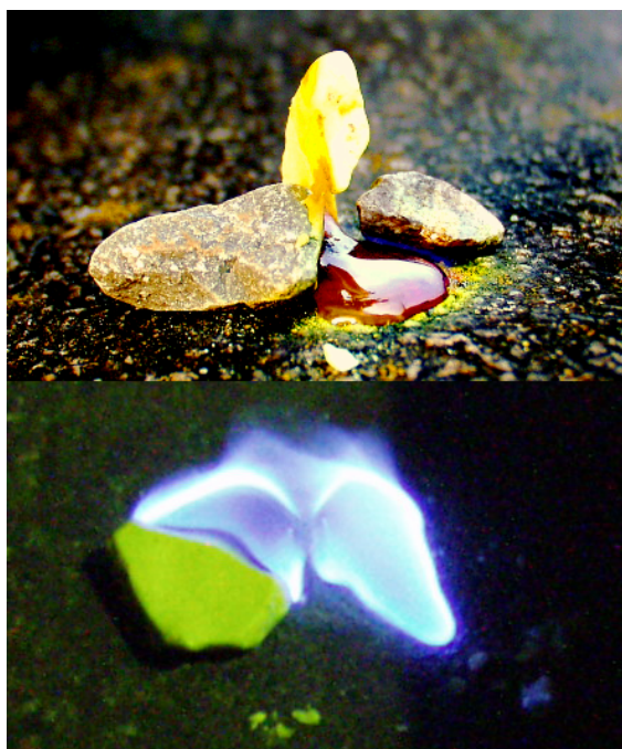
When burned, sulfur melts to a blood-red liquid and emits a blue flame that is best observed in the dark.
