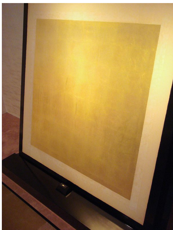
A gold nugget of 5 mm in diameter (bottom) can be expanded through hammering into a gold foil of about 0.5 square meters. Toi museum, Japan.
