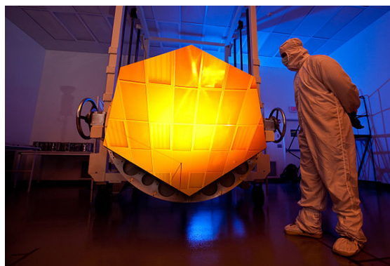
Mirror for the future James Webb Space Telescope coated in gold to reflect infrared light
