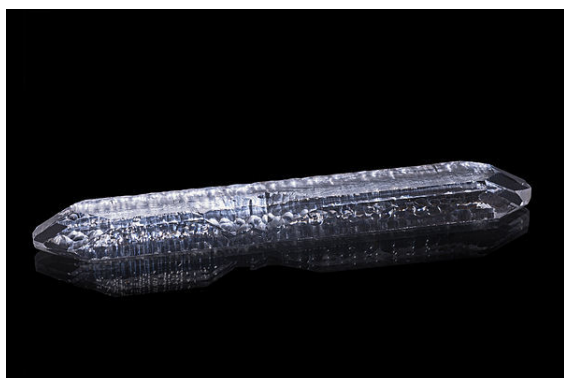
A synthetic quartz crystal grown by the hydrothermal method, about 19 cm long and weighing about 127 grams
